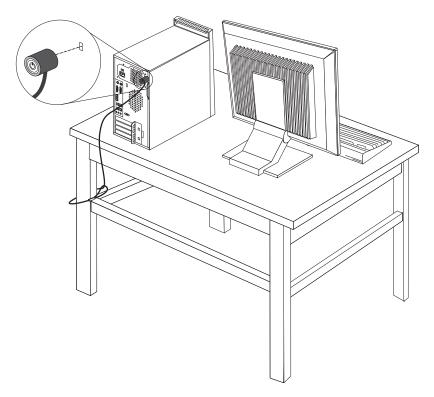
Figure 40. Integrated cable lock
